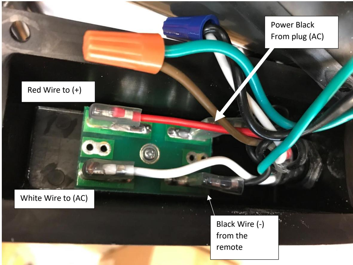
On the bridge rectifier in the photo above, black wire coming from the plug connects to the red wire side.
